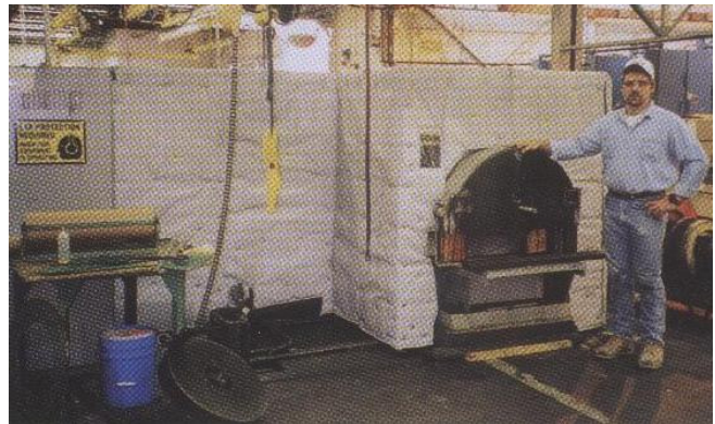
Metal Framework & Custom-Built Sound Enclosure Design: LT250A-VP-1.5” Thick 10.3 dBA Reduction
